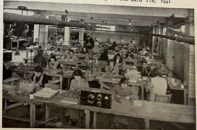
ASSEMBLING EDDYSTONE RECEIVERS IN FORMER LADIES' DRESSING ROOMS
