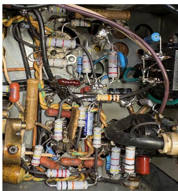
Above: the BFO/AM detector/noise limiter/1 st audio and audio output section of the chassis (left – before refurbishment, right – after refurbishment). Below: close-ups of the same
