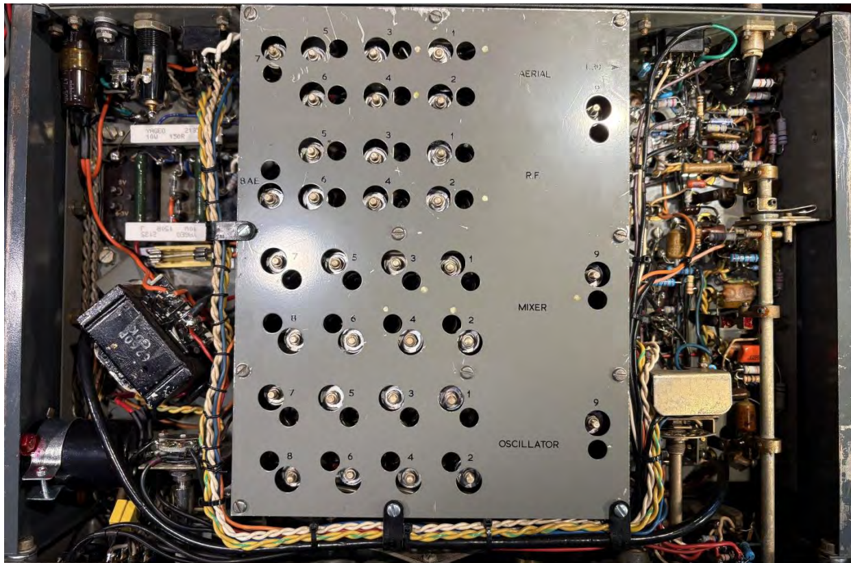
Above: underside of the chassis after refurbishment (with coilbox cover installed). Below: the refurbished set on soak test – performing well!
