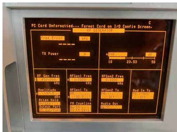
Above left: SNR on Band 7 (450KHz) = >23dB
