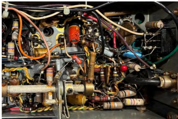
Above: the BFO/AM detector/noise limiter/1 st audio and audio output section of the chassis (left – before refurbishment, right – after refurbishment). Below: close-ups of the same
