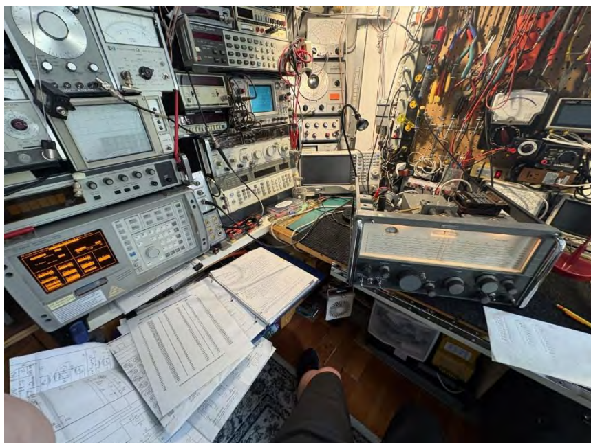
Right: Test set-up for making SNR measurements with the Agilent 8935 E6380A CDMA Test Set (located at the bottom left of the instrument stack)
