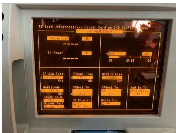
Above: SNR on Band 1 (24.0MHz) = &gt;18dB
