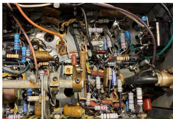
Above: the BFO/AM detector/noise limiter/1 st audio and audio output section of the chassis (left – before refurbishment, right – after refurbishment). Below: close-ups of the same
