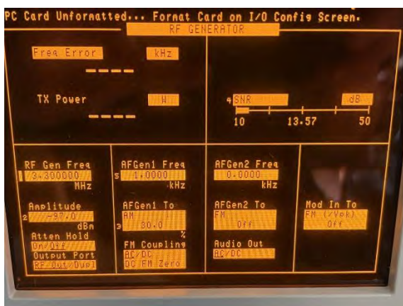
Above left: SNR on Band 5 (3.3MHz) = >13dB
