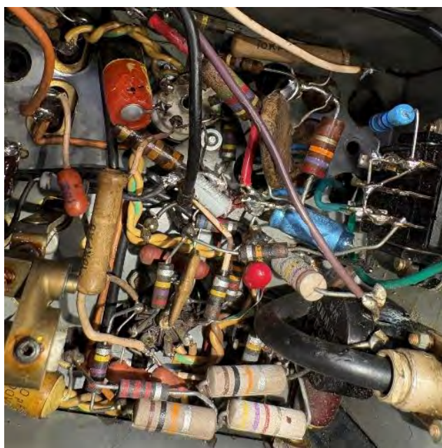
Above: the BFO/AM detector/noise limiter/1 st audio and audio output section of the chassis (left – before refurbishment, right – after refurbishment). Below: close-ups of the same
