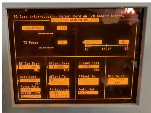
Above left: SNR on Band 3 (9.0MHz) = &gt;15dB
