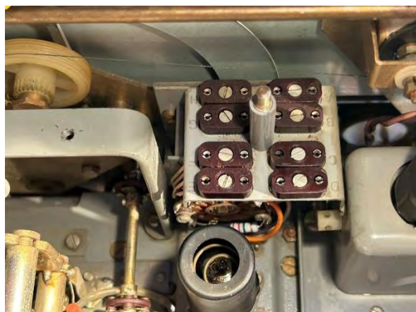
Left: Close-up of the audio stages and 100KHz IF cathode follower stage after rework. Below left: the 2 nd local oscillator/mixer compartment showing the crystal socket that can be used to fix the 2 nd local oscillator frequency. Below: 1 st local oscillator crystal bank
