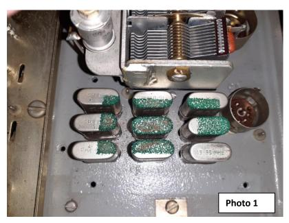
and the crystal cans were covered in corrosion. This is shown in Photo 1. Next, I examined all the mechanical aspects of the receiver, to check the operation of the controls and the state of the lubrication. All the controls appeared to be working correctly, although several felt a bit stiff, and there were still some signs of a little lubrication. I examined the main tuning mechanism very carefully; looking for possible causes of the
