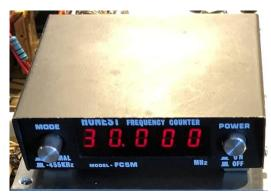
and hence providing direct readout of the tuned frequency of a set with a 455KHz IF tracking high of the signal frequency. I had tested the unit when it arrived from the UK, but had never got around to fitting the unit to a radio. It occurred to me that as my S.940 has a nominal IF of 455KHz (not the 450KHz as standard, as I used a 455KHz crystal for the crystal filter), it may be a good candidate to try this out on.
