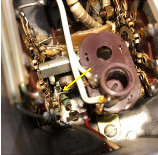
resistors and a silver mica capacitor that hindered access. Pin 7 (cathode) of the RF amplifier tube socket was now accessible. The photos, left, show access before (top) and after (below) better access was made. Pin 7 of the tube socket is marked with an arrow in both photos.
