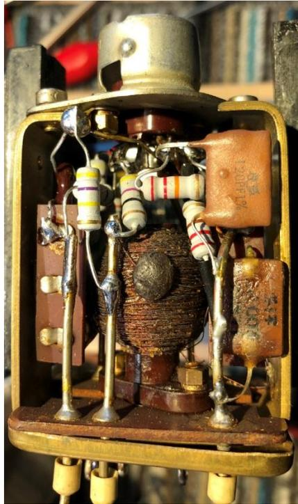
I replaced the IF filter caps with ones of the correct values and the coupling cap with a 0.047uF cap rated at 630vDC. The small electrolytic had been changed, for one of the correct value, and this checked out ok. Only one resistor had been changed-out (for one of an incorrect value). On testing the others, only one was significantly out of tolerance. However, I went ahead and replaced them all anyway – this will save time in the long-run as removing/replacing this unit is a bit of a pain. The
