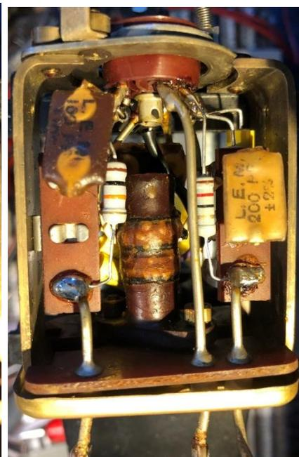
unit and fitting back into the chassis. It function tested ok once installed and wired-up. I noticed that one of the resistors that someone had replaced previously (the 27Kohm screen dropper connecting to the 2<sup>nd</sup> converter unit in the IF/AF compartment) was also an incorrect value, so I replaced that also.
