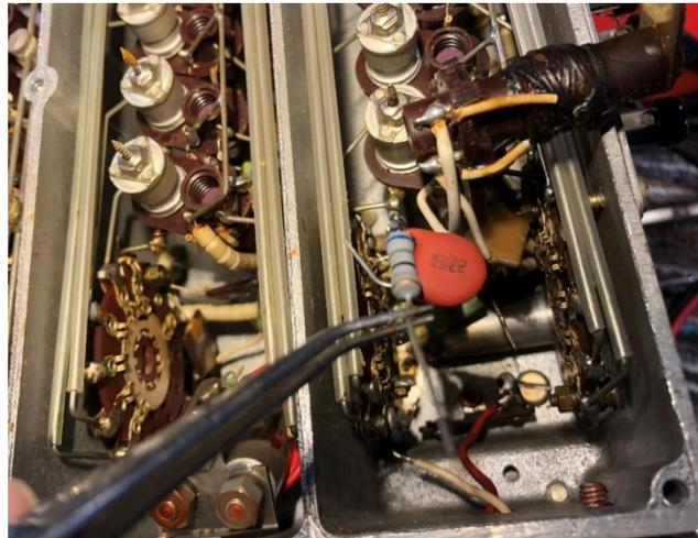
change out 4 components! – photo, below right) – worth it though as I noticed an improvement in RF gain after these changes.
