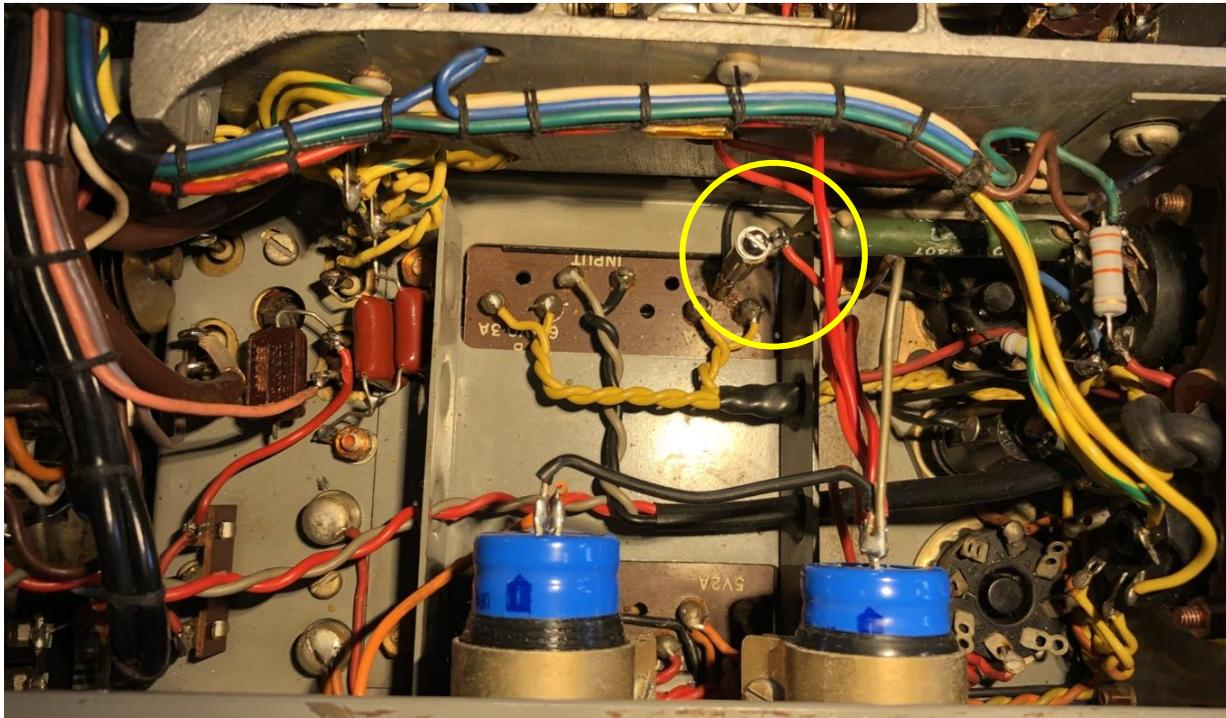
and I was 'in the mood'. This included installing an insulated standoff to support one end of the 2.7Kohm wire wound dropper resistor feeding the voltage stabilizer tube (circled in photo, above) – this had been left 'hanging in the breeze' after someone had replaced the filter caps. I also replaced a couple more resistors in the power supply chassis where they tested out of tolerance.
