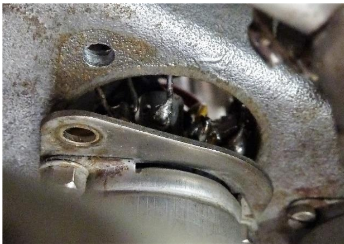
Figure 8: Rewiring tube socket from above
