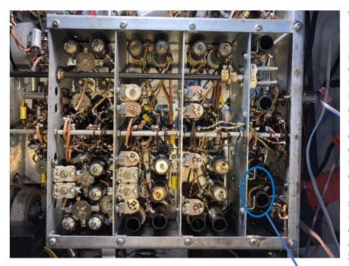
The RF deck of the Hallicrafters SX-28 and 28A are notorious for poor access to several capacitors and resistors buried deep (photo, left) - some are almost invisible looking directly down on where the component(s) is located, being obscured by the bandchange switch shaft and wafers, numerous wires and other components, and, in the case of the SX28A, SRPB boards.
