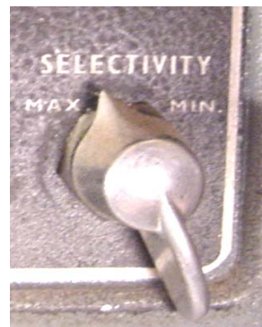
'No-frills' front panel control of selectivity on an S.750 – simple but very effective in use...
