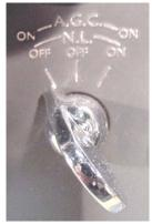
(usually resulting from impulse noise, such as 'static') off the signal - this can be very effective in making impulse-type noise become relatively inaudible, though is pretty-
