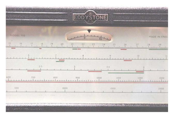
Above: the lovely linear 'sliderule' dial from my S.750 – the logging scale at the bottom is used in conjunction with the circular 'vernier' dial at the top to provide excellent frequency logging capability and reproducibility. Below: introduction to the Eddystone pamphlet 'Better Radio Reception' (1958 version)
