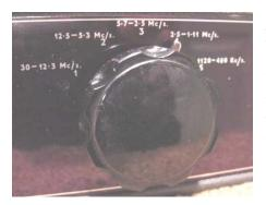
**Band Switch:** this is a multi-pole, multi-way switch, normally comprising several switch wafers, each mounted in a section of the diecast coilbox assembly. The switch connects the appropriate RF, mixer and oscillator coils into the circuit for each band selected and usually simultaneously shorts the unused coil units to earth, thus preventing unwanted parasitic resonances from absorbing RF energy from the tuned circuit actually in use.
