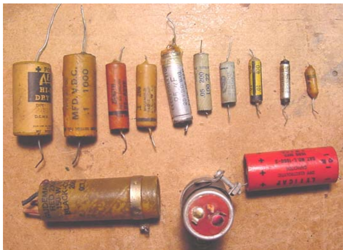
A selection of 'failed' caps removed from valve radios (alas, not all Eddystones...)
