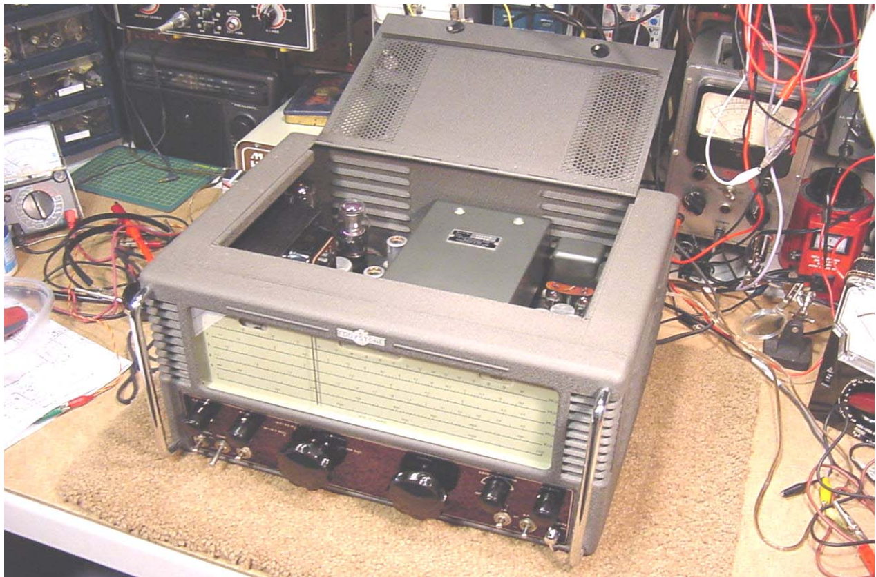
Below: the S.680X on the G8GUH workbench following re-assembly and undergoing soak-testing
