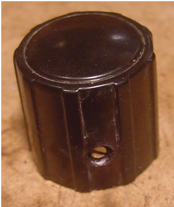
Above left: Over-sized hole re-shaped into a hexagonal shape and 6BA nut inserted from inside the knob. Above: 6BA screw with heatshrink sleeve threaded into the nut. Left: Repaired knob with 6BA grub screw installed
