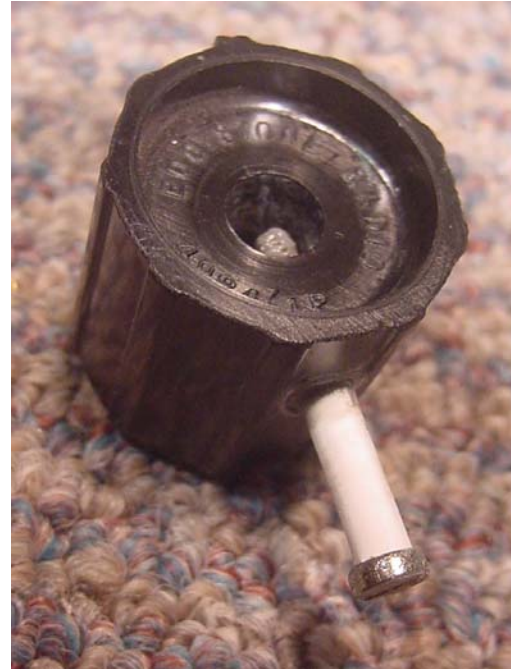
Above left: Over-sized hole re-shaped into a hexagonal shape and 6BA nut inserted from inside the knob. Above: 6BA screw with heatshrink sleeve threaded into the nut. Left: Repaired knob with 6BA grub screw installed
