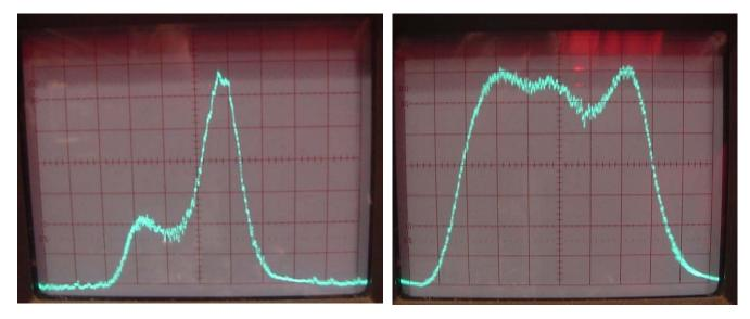
Above left: widest AM setting before adjustment – oh dear, what a camel back! (or cross-section through the Matterhorn?). Above, right: widest AM setting after adjustment – not perfect, but looks much better with a 6kHz bandwidth at -6dB (and better-sounding too)
