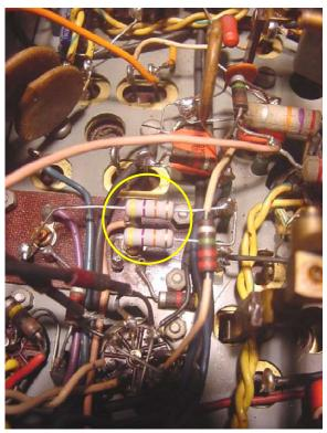
found to drift high as it was warmed up with a hair-dryer. I changed these resistors for metal-film 1 Watt types (photo, base of previous page) in both the USB and LSB circuits. Problem solved – I now had the full range of adjustment back and no drifting on LSB.
