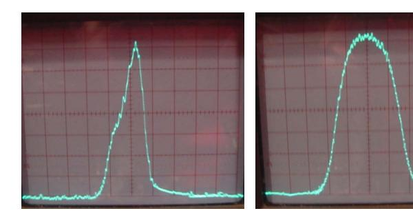
Above, left: SSB setting before adjustment – too sharp at the nose and some asymmetry creeping in (start of the hump forming on the low-frequency side). Above, right: SSB setting after adjustment – flatter top, around 2.4kHz width at -6dB, symmetrical and steep skirts
