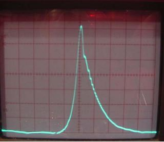
Above, left: crystal setting before adjustment – note the pronounced 'ringing' and very asymmetric shape. Above, right: crystal setting after adjustment – now much sharper, with a very distinct peak and a bandwidth of around 200Hz at -6dB, coupled with less ringing and less asymmetry
