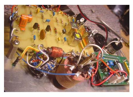
in the wobbulator's voltage controlled oscillator (VCO) could be made to swing the VCO sufficient to cover the receiver IF passband at this low frequency – this was later checked and found to be more than adequate. Having completed the experimentation and having confidence in my selection, I fitted the coil into the wobbulator. It was a rather neat fit, but I managed to squeeze it in (just) between the 'Range' and 'Counter' rotary switches (photo, above).
