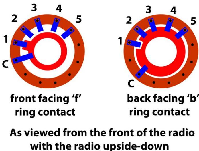
The inner ring is the moving contact on both sides of the switch; they are of course 'ganged' together to move as one but they are insulated from one another.
