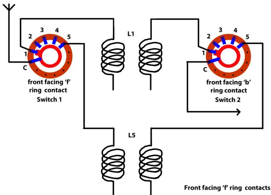
Note that in each section the highest frequency's coils are positioned nearest to the wafer switch.
