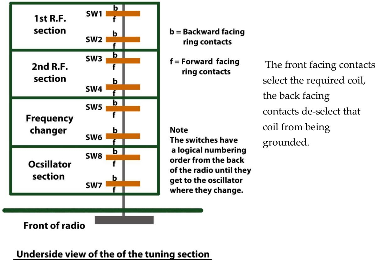
All eight of the wafer switches of the band change are identical.
