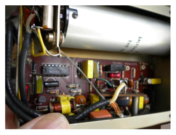
Now we can see the GEC temperature controlled crystal osc in its long can along with the divide by 10 circuit and pulse circuits.
