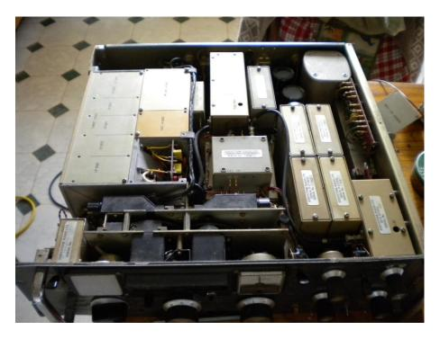
This receiver was obtained from a clear out at a local radio club as being totally not working at all. Subsequent examination and basic repairs got the basic set working but not the Stabilised loop system used on ranges 1-4 ie 1.6 Mhz to 30 Mhz.
