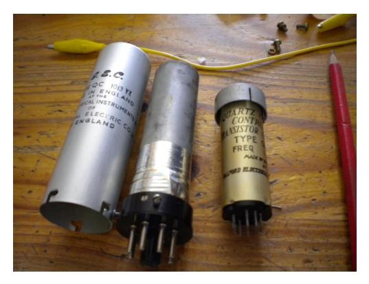
Now in my case the pins to the 9 pin B9A socket were badly oxidised so hopefully a good clean will get it working but NO it didn't . So investigation further deeded. With a small screwdriver ease up the 4 crimps about the base of the inner can.
