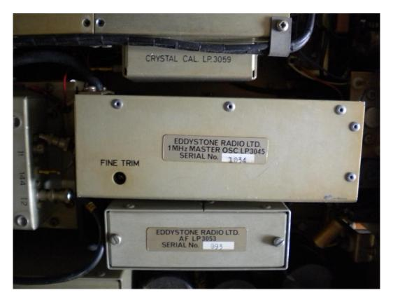
Now the master Osc unit looks formidable however after examining the manual there are only four voltage connection and two RF outputs.
