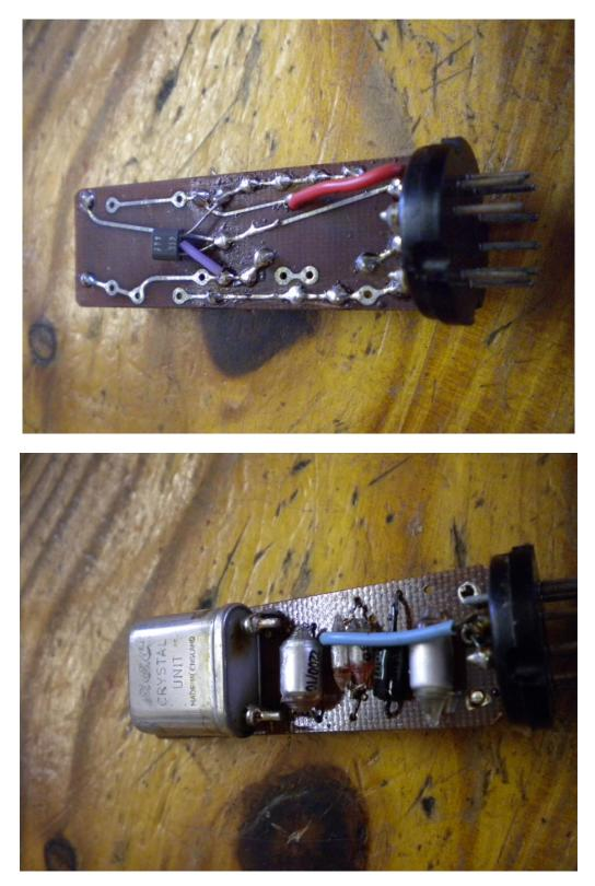
This will allow you to see the simple PCB within the 1 Mhz Crystal PCB and a ZTX312 transistor . Examination of the components will identify the fault which in my case turned out to be the larger 2200pf polystyrene capacitor had gone short circuit and the 100 K resistor at the top was 174k. Both were replaced and the unit tested with success.
