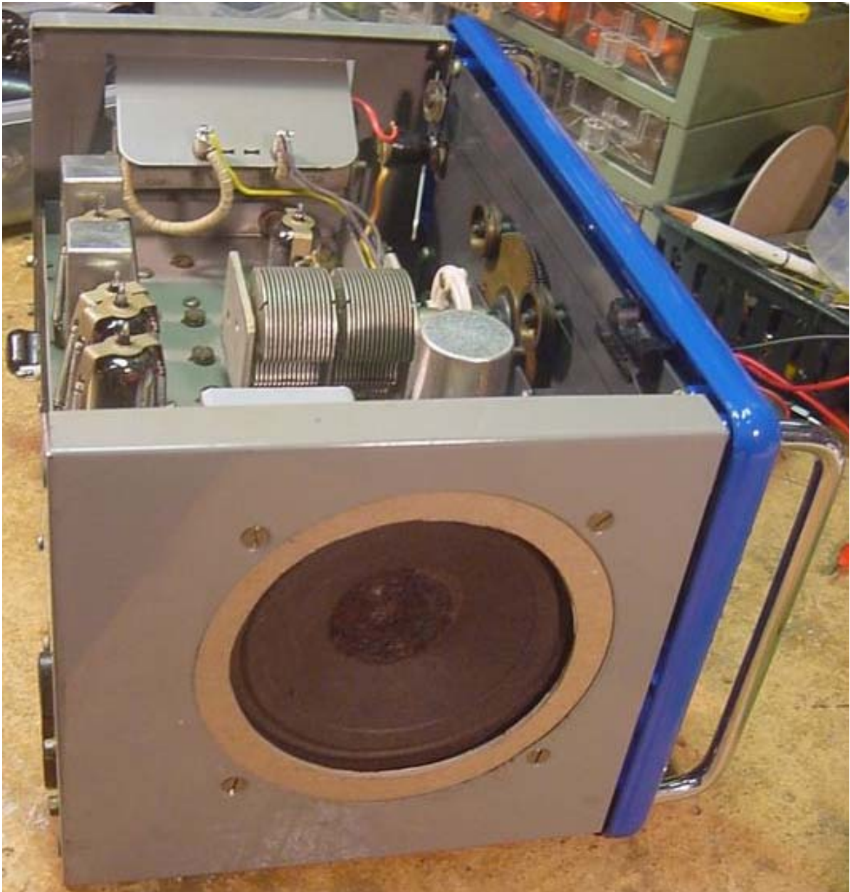
Above: replacement speaker fitted into the S.870
