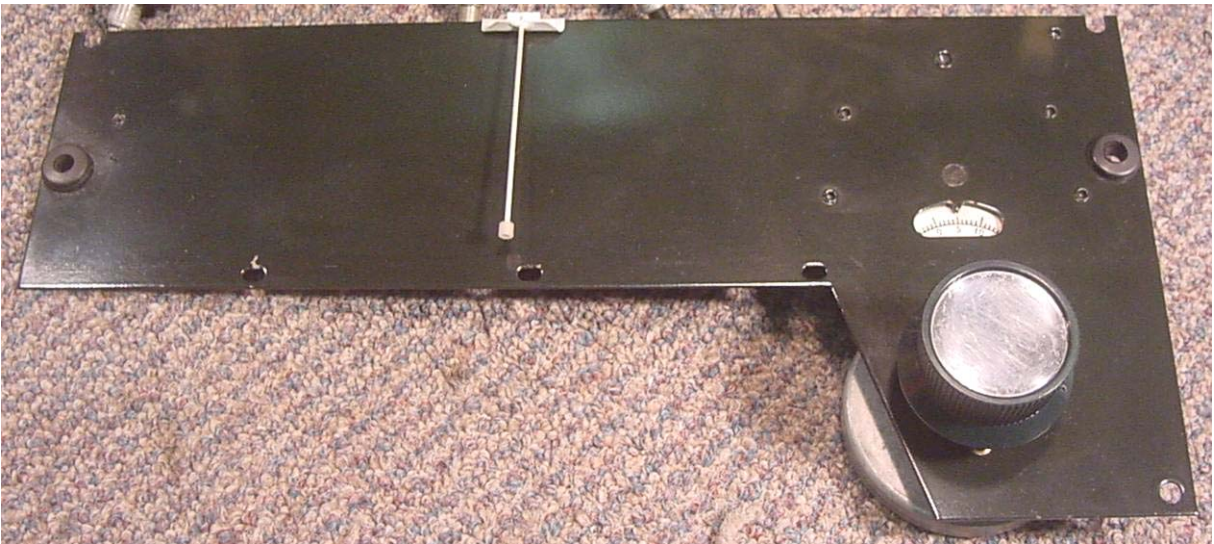
Above/below: the tuning mechanism removed from the set. The main issues here were a dirty friction clutch and a distorted idler pulley (on right, below)
