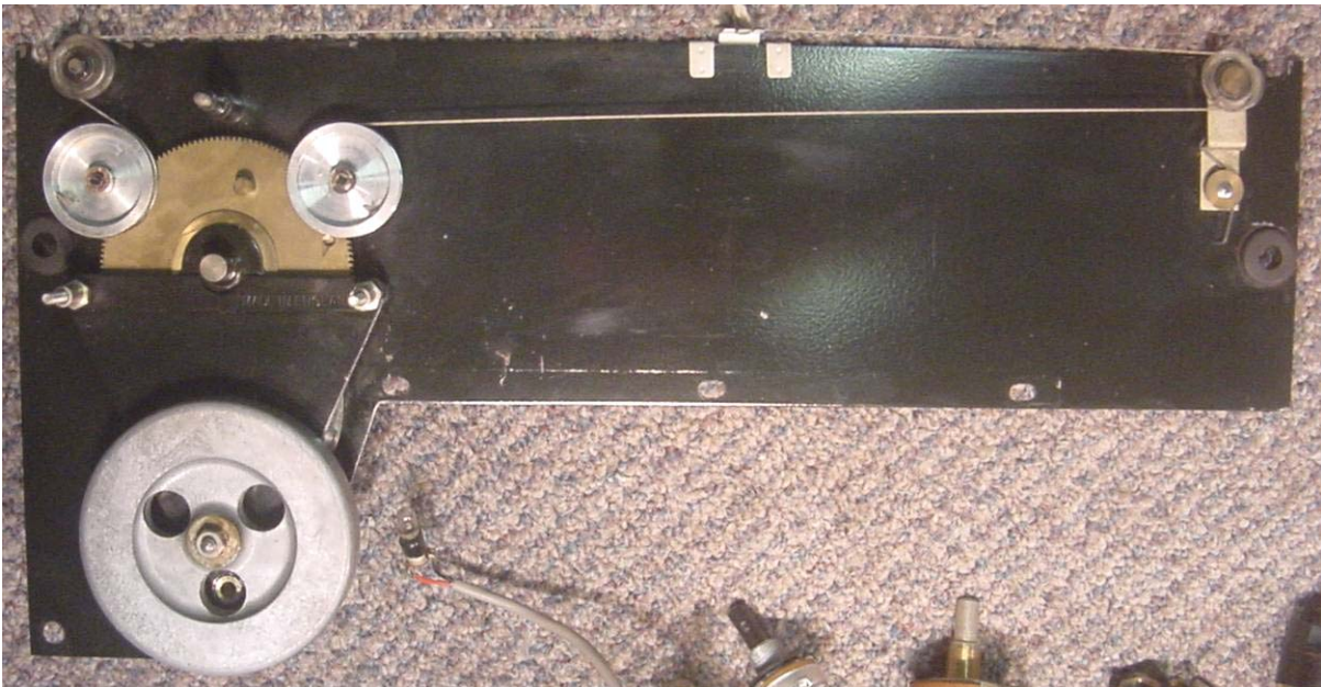
Above/below: the tuning mechanism removed from the set. The main issues here were a dirty friction clutch and a distorted idler pulley (on right, below)
