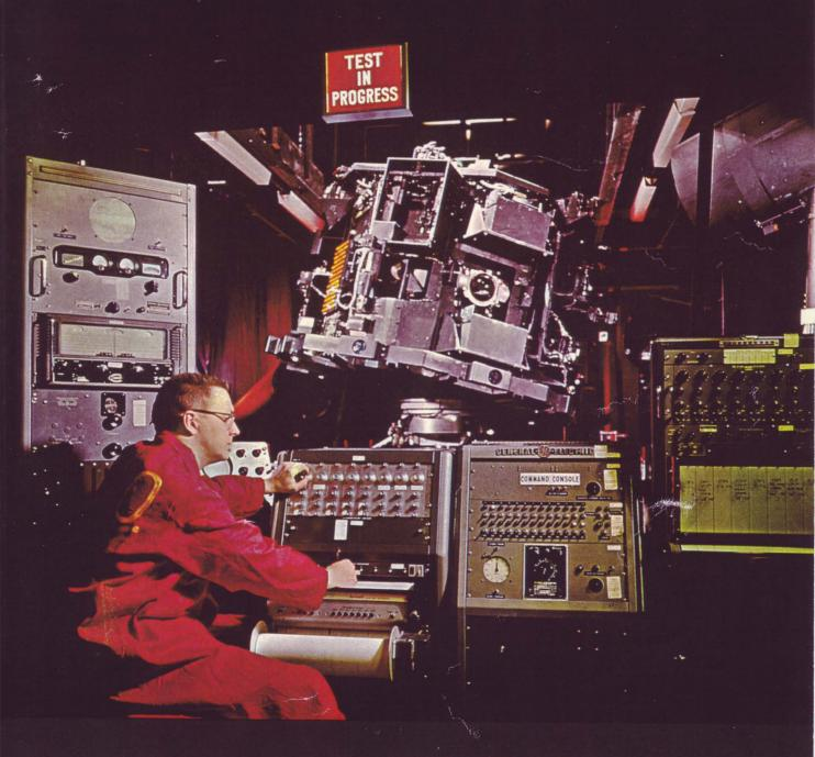
STABILIZATION AND CONTROL SYSTEM for the NASA Orbiting Astronomical Observatory is undergoing static test in a dynamic balancing facility at General Electric's Missile and Space Div. Valley Forge facility. Because the star tracker is operating, no white light source can be used. But the tracker is not sensitive to the red light, which is used here for illumination and casts the purplish glow over the instrumentation.
