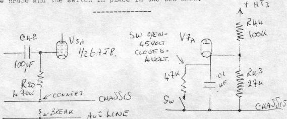
R20 is disconnected from the AVC line and connected to earth.
