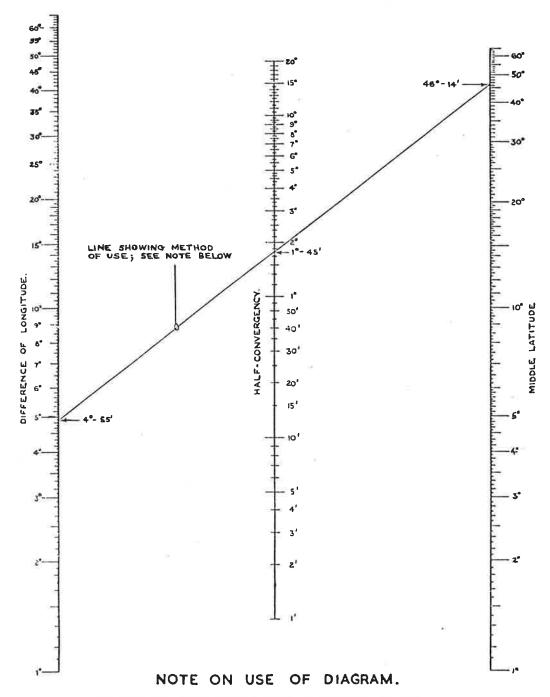
TO FIND THE HALF-CONVERGENCY IN RESPECT OF TWO PLACES, THE DIFFERENCE IN LONGITUDE OF WHICH IS 4"-55' AND THE MID-LATITUDE 46"-14", PLACE A STRAIGHT EDGE IN THE POSITION SHOWN, SO AS TO INTERSECT THE OUTER SCALES AT THE GIVEN POINTS, AND READ OFF THE HALF - CONVERGENCY 1"-45" ON THE CENTRE SCALE.
