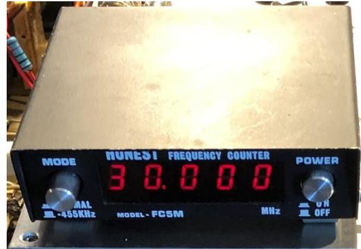
and hence providing direct readout of the tuned frequency of a set with a 455KHz IF tracking high of the signal frequency. I had tested the unit when it arrived from the UK, but had never got around to fitting the unit to a radio. It occurred to me that as my S.940 has a nominal IF of 455KHz (not the 450KHz as standard, as I used a 455KHz crystal for the crystal filter), it may be a good candidate to try this out on.
