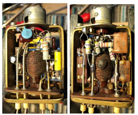
I replaced the IF filter caps with ones of the correct values and the coupling cap with a 0.047uF cap rated at 630vDC. The small electrolytic had been changed, for one of the correct value, and this checked out ok. Only one resistor had been changedout (for one of an incorrect value). On testing the others, only one was significantly out of tolerance. However, I went ahead and replaced them all anyway – this will save time in the long-run as removing/replacing this unit is a bit of a pain. The
