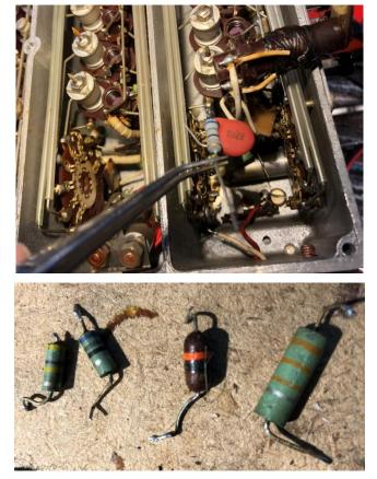
5000pF audio coupling cap with a 0.01uF part rated at 160vDC. This cap has 200vDC on it from the anode of the product detector tube, so not good... The larger IF bypass caps would account for slightly dull-sounding audio during SSB reception.
