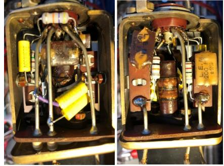
unit and fitting back into the chassis. It function tested ok once installed and wired-up. I noticed that one of the resistors that someone had replaced previously (the 27Kohm screen dropper connecting to the 2<sup>nd</sup> converter unit in the IF/AF compartment) was also an incorrect value, so I replaced that also.
