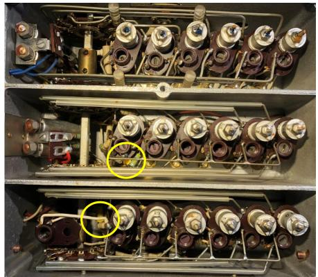
performance. So I changed these three bypass caps out: two in the coilbox and moderately difficult to access – circled yellow in photo, above, and one in the IF compartment and much easier as noted earlier, circled green in the photo at the bottom of page 2.
