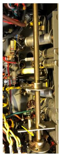
trim tool fashioned from a plastic knitting needle as my usual trim tools would not quite pass through the components and IF bandwidth control shaft above the core access hole (arrow on photo, above right).
