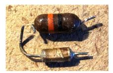
almost zero. I think their ageing behaviour depends on many factors – including manufacturer, batch, and environmental conditions. Examining the AF/IF compartment again revealed another such cap (AGC bypass on the 2<sup>nd</sup> converter tube), connected across a couple of pins on the 1<sup>st</sup> IF transformer. Checking the schematic, I identified that there were likely a few more of these types in the above-chassis Product Detector and 2<sup>nd</sup> converter units.
