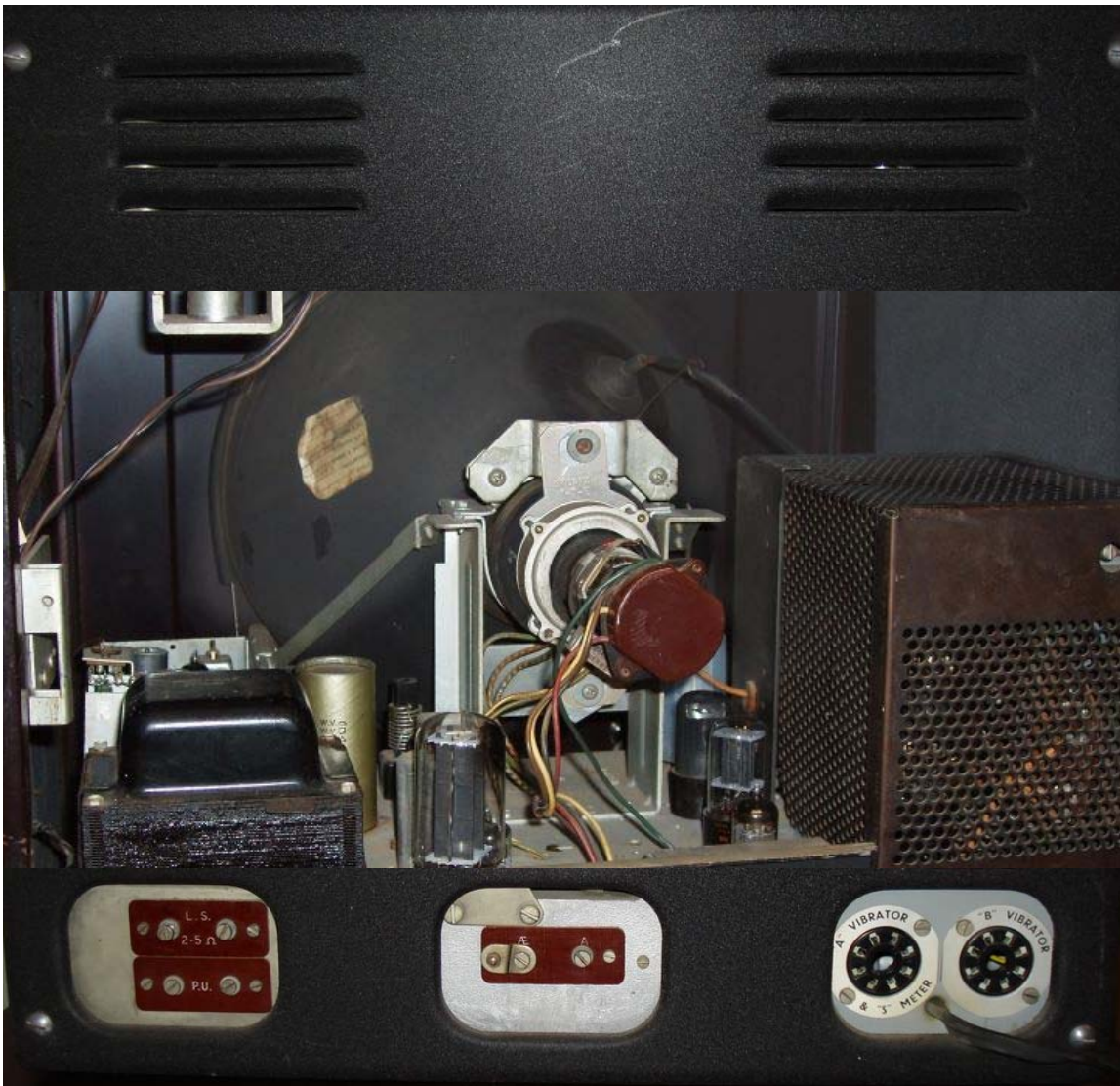
Above: View through rear panel – note Vibrator/S-Meter connector and pick-up input
