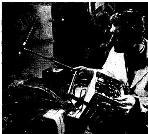
Fig. 5. The measuring set being used to trace a noise source
