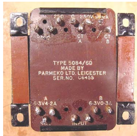
Mains transformer from an S.750 (Eddystone Part #3937P, aka Parmeko Type 5084/6D)... or was that from an S.770R,... or even an S.940?
