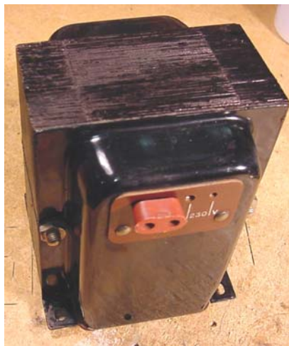
Mains transformer from an S.750 (Eddystone Part #3937P, aka Parmeko Type 5084/6D)... or was that from an S.770R,... or even an S.940?
