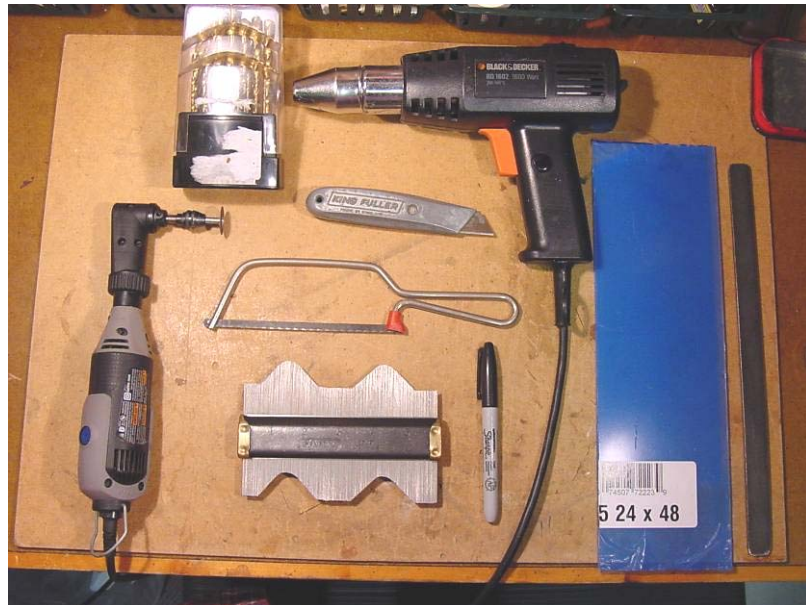
Tools of the Perspex-case maker: the template shows the actual outer radius of the case corners (S.740's case) on the left and that of the Perspex case corners on the right.
