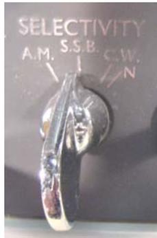
the other involved the switching of a tertiary coil(s) in/out of circuit in one or more of the IF transformers, as in the S.940. Some sets, eg. the S.680X, automatically adjust the receiver IF gain with selectivity in order to help equalise receiver output when varying the selectivity. Both of the variable selectivity methods used by Eddystone result in very effective and useful controls. See the Tech Short on Crystal Filters and Receiver Selectivity for more discussion on this subject.
