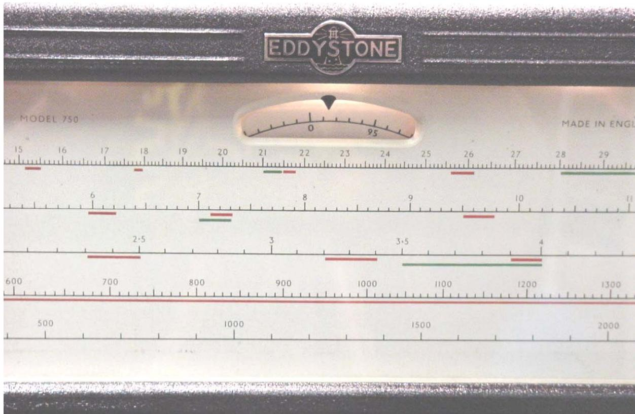
Above: the lovely linear 'sliderule' dial from my S.750 – the logging scale at the bottom is used in conjunction with the circular 'vernier' dial at the top to provide excellent frequency logging capability and reproducibility. Below: introduction to the Eddystone pamphlet 'Better Radio Reception' (1958 version)
