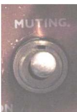
**Mute:** usually only found on sets designed for FM reception, this control activates a circuit that silences the receiver when the received signal is below a pre-determined threshold level. Sometimes the threshold is adjustable by the operator.
