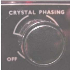
behaviour of which may be adjusted using the 'phasing' control to provide either a peak in the received signal or a null ('trough' or 'slot') at a slightly offset frequency – these facilities are very useful for CW reception (see below). Again, the interested reader should refer to the Tech Short on Crystal Filters and Receiver Selectivity for more discussion on this subject.
