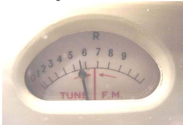
NBFM can be received (after a fashion) on sets without a discriminator, using the 'slope detection' technique. To do this, the receiver is set up as for AM reception and the tuning slightly offset (by around half the bandwidth of the NBFM signal) to one side or other of the signal. At this point, variations in frequency of the received signal caused by the original modulation will result in amplitude variations as the signal frequency moves across the slope
