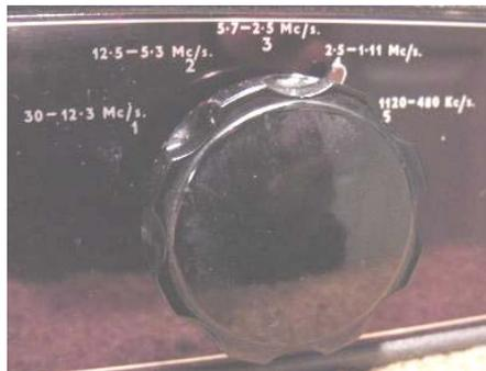
**Band Switch:** this is a multi-pole, multi-way switch, normally comprising several switch wafers, each mounted in a section of the diecast coilbox assembly. The switch connects the appropriate RF, mixer and oscillator coils into the circuit for each band selected and usually simultaneously shorts the
