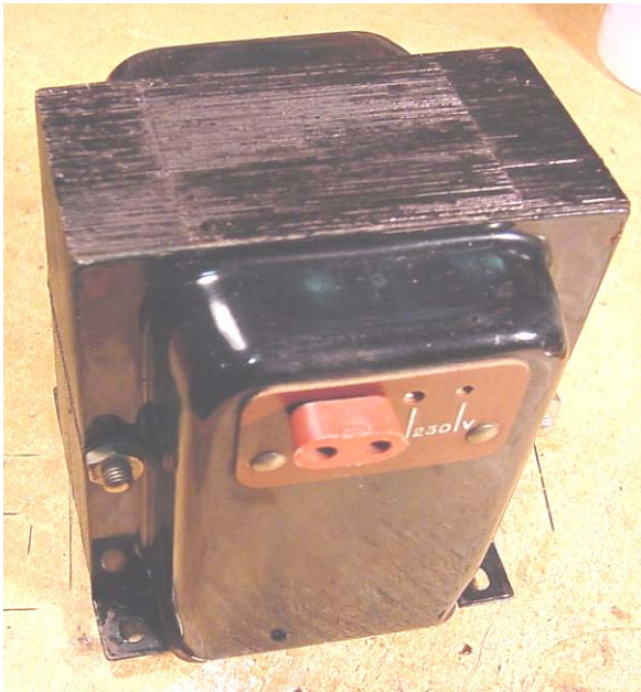
Above: Parmeko Ltd. power transformer Type 5084/6D, alias Eddystone Part No. 3937P. This same transformer type was used in several Eddystone valve receiver models from the early 1950's (eg. S.750) through the early 1970's (eg. S.940)
