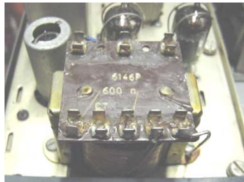
Push-pull audio output transformer from an S.940. Note the 600 ohm line output
