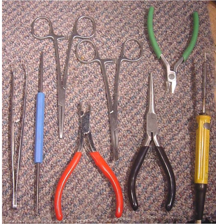
Above: Selection of tools suitable for working in politicians mouths er, I mean S770U AF compartments – hemostats (straight and curved), locking tweezers, long-necked cutters, needle-nosed pliers, angled soldering pick and that all-important 15W Antex soldering iron (this baby is 38 years old – well the handle is at least...)
