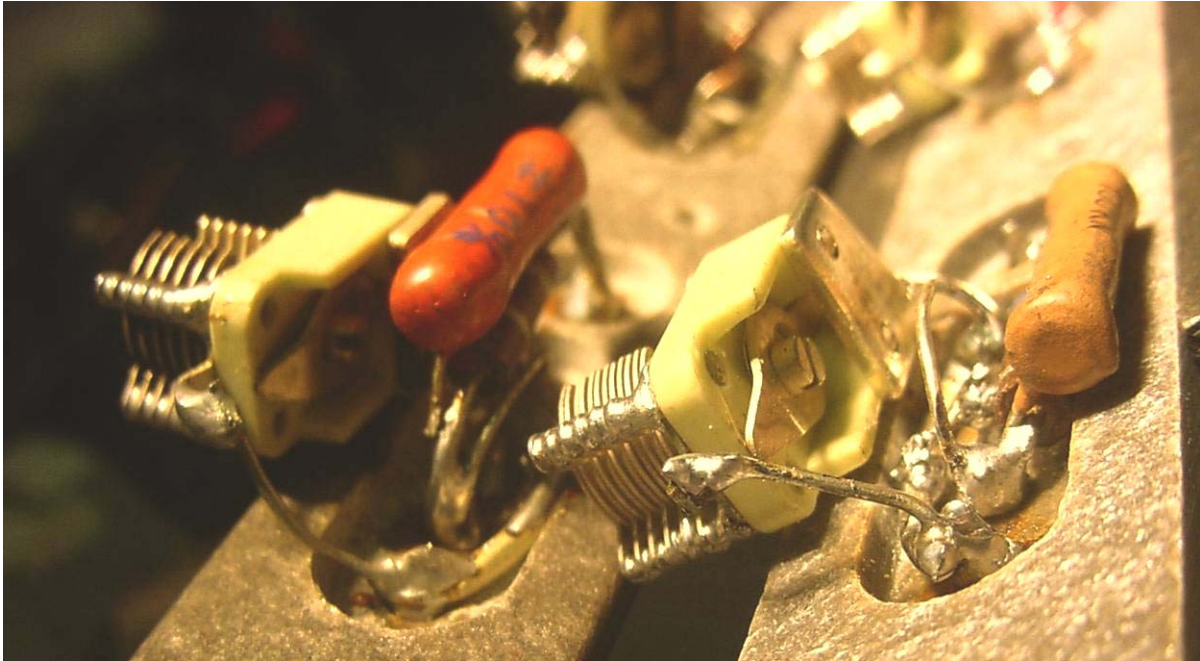
Above: Close-up of the Range 2 RF tuned-circuit under construction (re-manufactured one to the right). Below: The Range 1 RF tuned circuit under construction (the re-manufactured one below)
