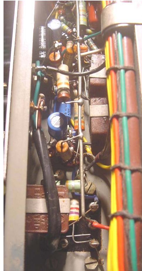
Above: The AF compartment after replacement of electrolytic capacitors (black and blue cases) – a bit like my fingers and the air in my shack after the work... (only kidding)
