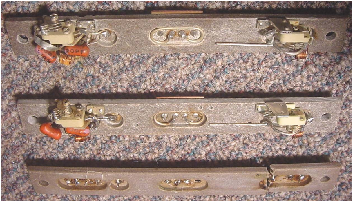
Above: the Range 1 biscuit from the SPARC Museum set (top), my re-manufactured Range 1 biscuit (centre) and the stripped-down broken Range 1 biscuit (bottom)
