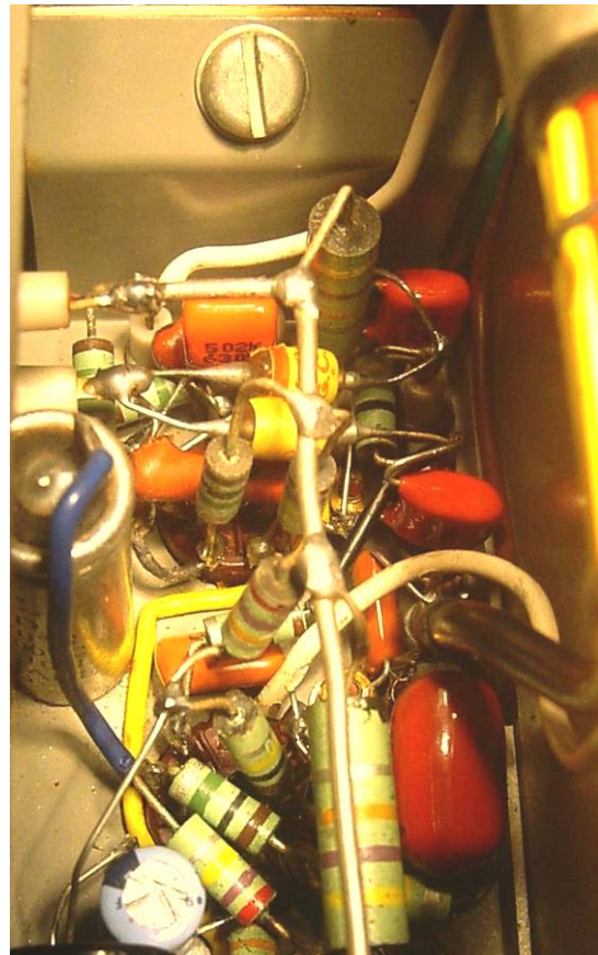
Above: The muting and first AF stages after replacing 'Rat Droppings' capacitors. Access is, to say the least, a little restricted...
