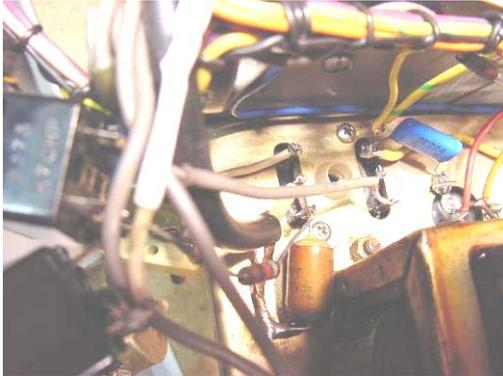
First I removed the can from the BFO unit and did some cursory component and pin-out checks before refitting it to the chassis and re-wiring into the circuit. While I had the opportunity I checked C72 (metallised paper heater decoupler) and found it to be leaky – replaced it (blue capacitor in photo, left).
