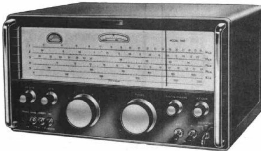
The EDDYSTONE Model 940 is a general purpose communications receiver covering the frequency band 480 kc/s to 30 Mc/s in five switched ranges. A single conversion circuit is employed and the receiver is suitable for AM, CW and SSB reception. A built-in mains pack provides for direct operation from all standard AC supplies.
