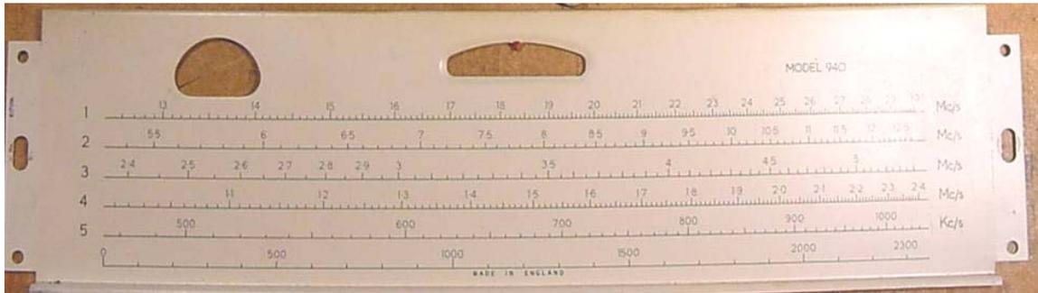
Vernier scale and main dial plate – the former looking a bit sad before cleaning...
