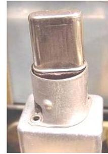
Of course I needed to re-align the IF in the set to 455kHz in order to use the crystal.
