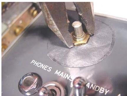
Removing the controls – note the oversized scratch guard
