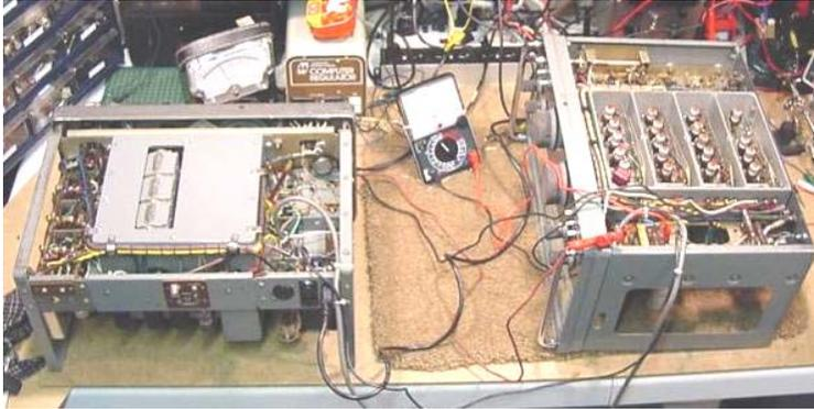
110mA HT and the 5Z4 at 125mA. I backed-off the applied AC voltage to give a current draw of 110mA (this being at about 105v AC), resulting in an HT2 voltage of only 225v.
