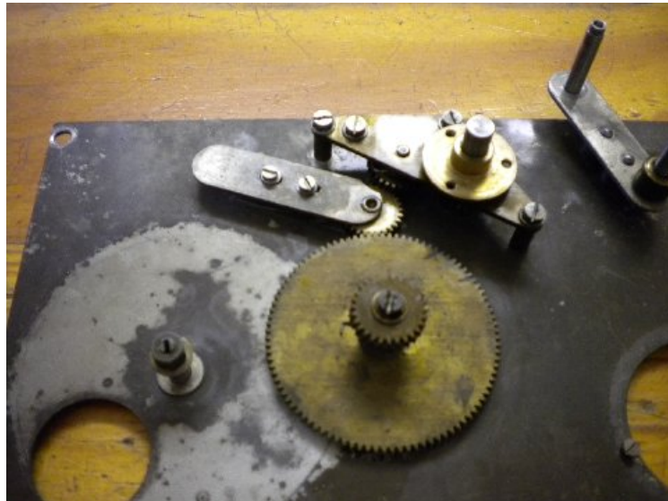
Photo 5. Idler gear fitted
