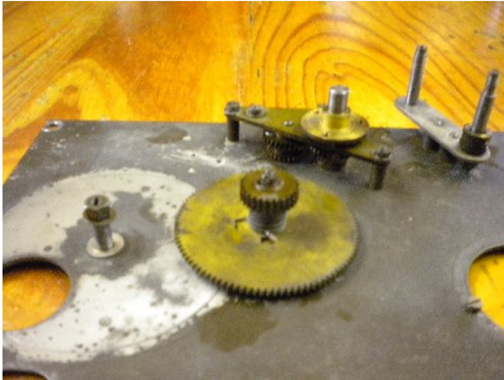
Photo 4. Large brass gear replaced
