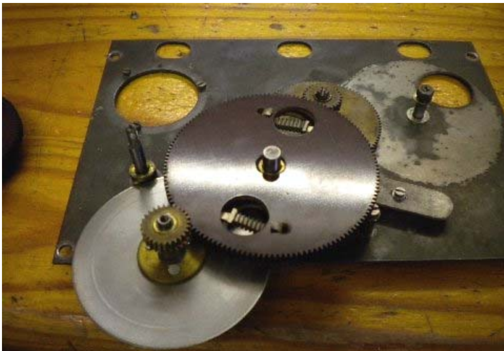
Photo 9. Final pointer drive wheel re-fitted
