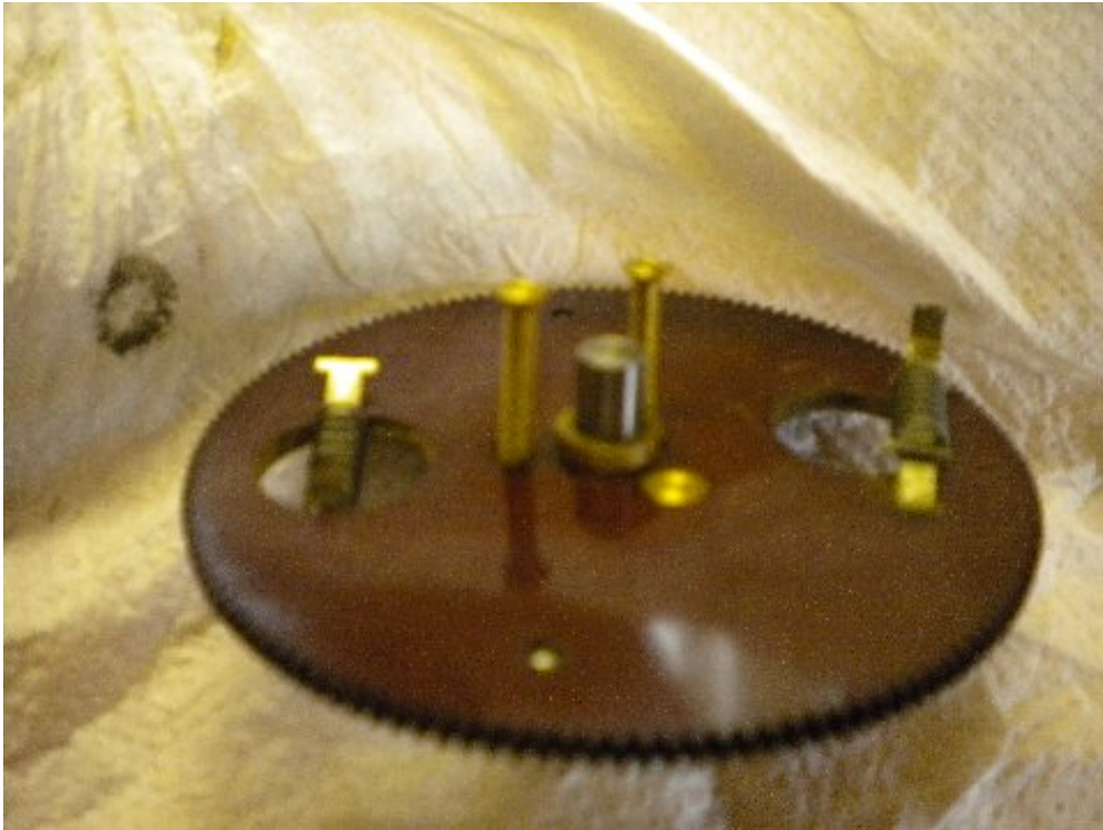
Photo 8. The large Paxolin drive wheel is in two halves - the lower half is screwed to the brass boss with three very small screws and they are each only holding by one turn. One of mine was stripped causing the wheel to run untrue, so three new brass 6BA screws were fitted and sawn off at the back . The thread was re-tapped as well.
