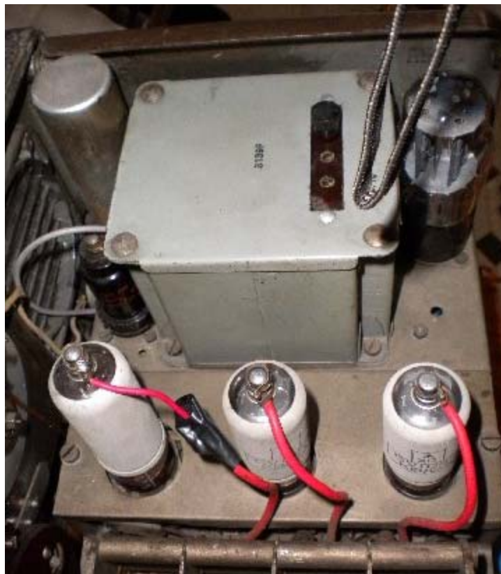
Photo 21. Power supply and RF stages
