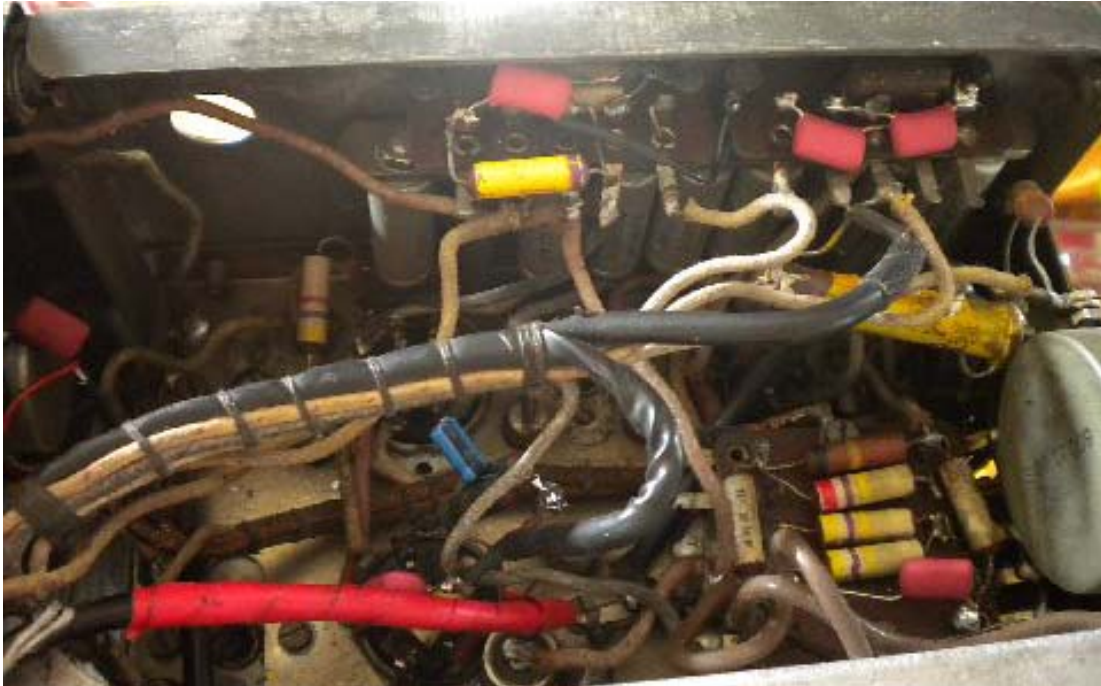
Photo 18. Re-capped IF section
