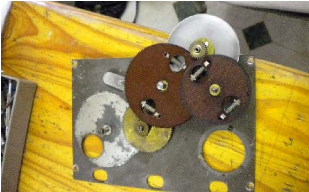
Photo 10. Six hands required for this one (see Photo 23). First the large final Paxolin drive wheel has to be tensioned and held. Then the smaller Paxolin drive wheel has to be tensioned and held. It is then slid down its shaft linking the spring steel wheel to the final drive. Once in place the anti-backlash springs can be released to take up the slack.
