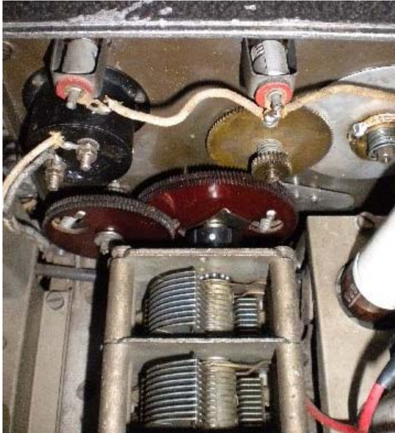
Photo 14. Dial drive mechanism installed in the S.504
