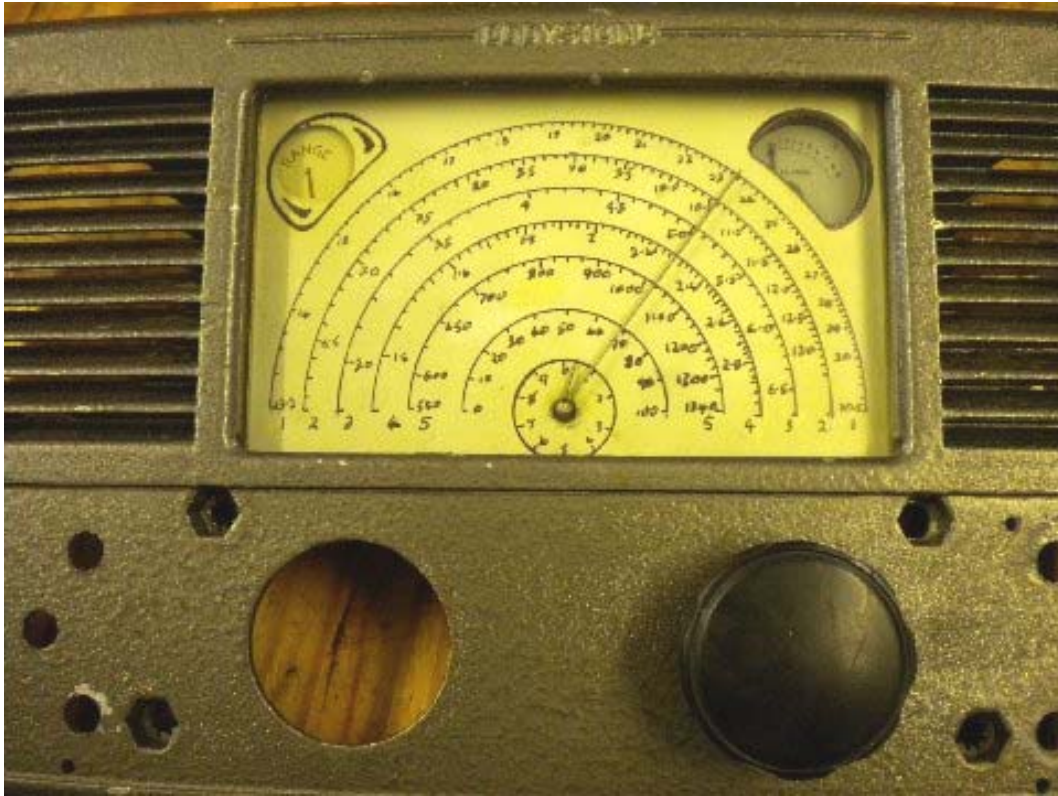
Photo 12. Front panel showing new hand-marked dial and testing the overhauled gear drive mechanism
