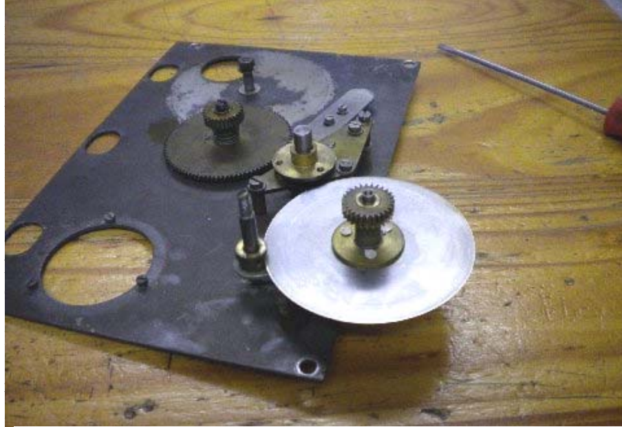
e Photo 6. Spring steel drive wheel and collar fitted.
