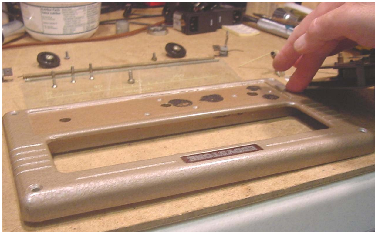
Above: Notice the slightly warped front panel casting – discussed in the text. Below left: yes, I finally invested in some BA nut runners. Below right: The tuning capacitor gang after being ‘Silvo’d’. Note the glass bead forming the rear shaft bearing (bottom of photo)
