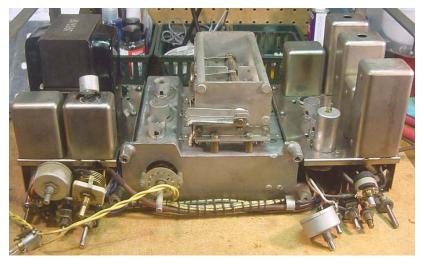
Other components were found to be within tolerance and valve voltages tested ok when 110v AC was applied to the set (unfortunately mains power on
