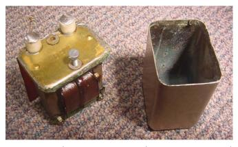
This 5.750 was not working on arrival due mainly to an open-circuit HT choke, now repaired: the fault was a corroded wire internally on one of the connection posts. I found that the choke can
