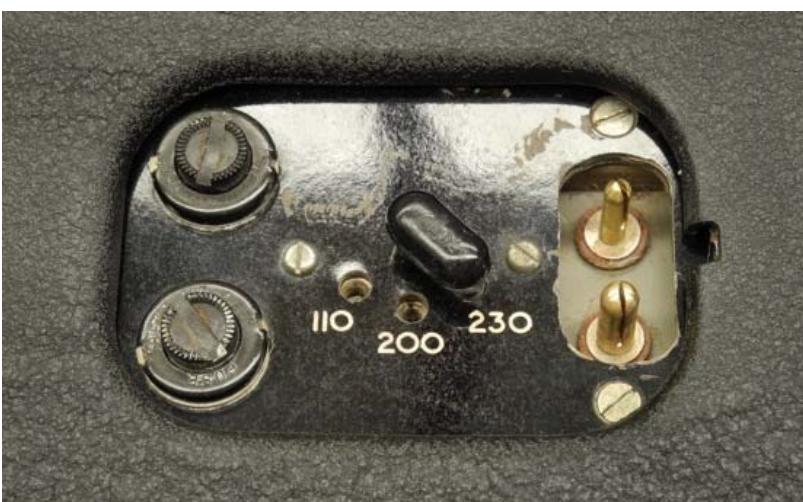
Left: Bakelite panel on the S.840A showing saddle with new pins and access hole straightened out
