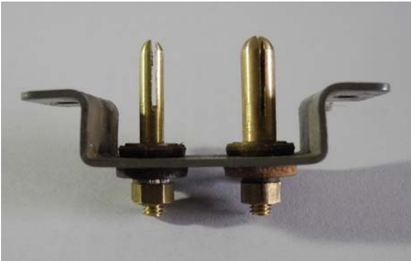
Left: original Eddystone mains input saddle with new pins to suit the Marquis plug - side view
