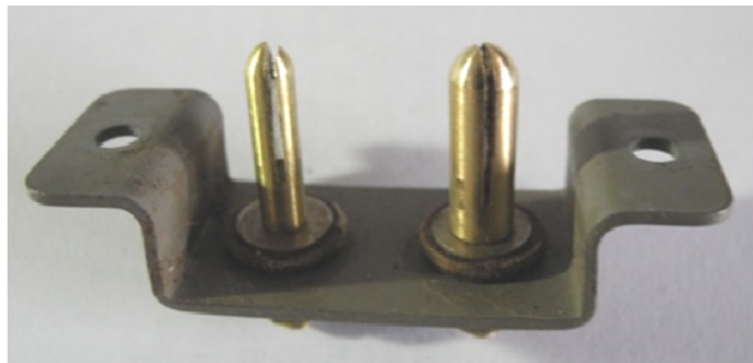
Original Eddystone mains input saddle with new pins to suit the Marquis plug oblique view
