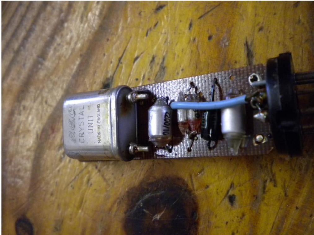
This will allow you to see the simple PCB within the 1 Mhz Crystal PCB and a ZTX312 transistor . Examination of the components will identify the fault which in my case turned out to be the larger 2200pf polystyrene capacitor had gone short circuit and the 100 K resistor at the top was 174k. Both were replaced and the unit tested with success.
