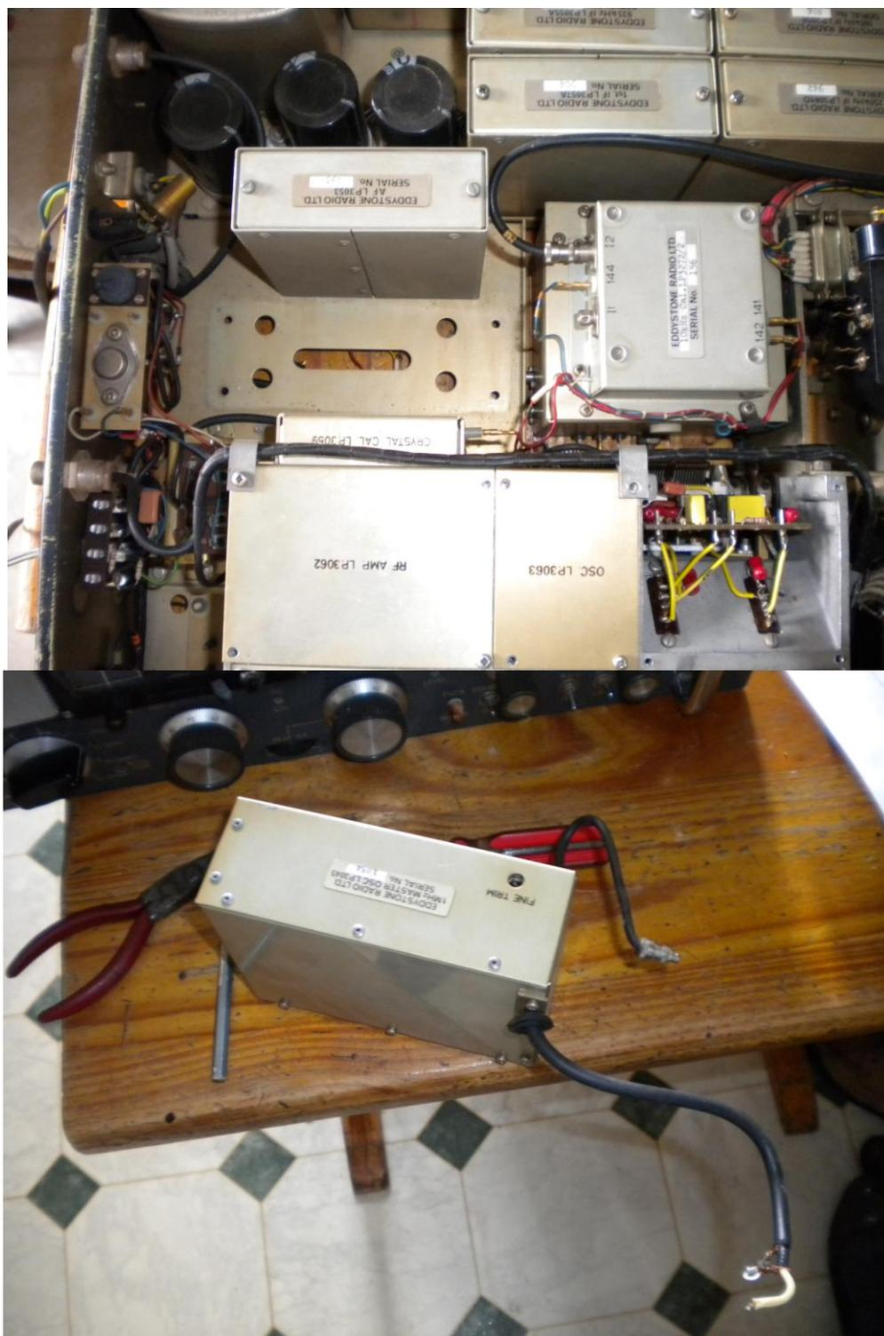
With the unit in my hands the main receiver chassis was removed to leave the bench(Kitchen Table ) free to work on the module. To provide power for testing a 12 gell battery was used and a set of Crock clip leads.
