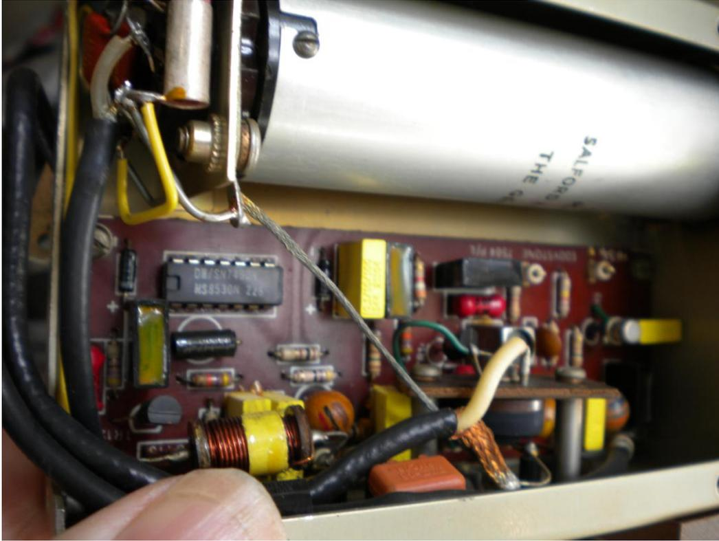
Now we can see the GEC temperature controlled crystal osc in its long can along with the divide by 10 circuit and pulse circuits.
