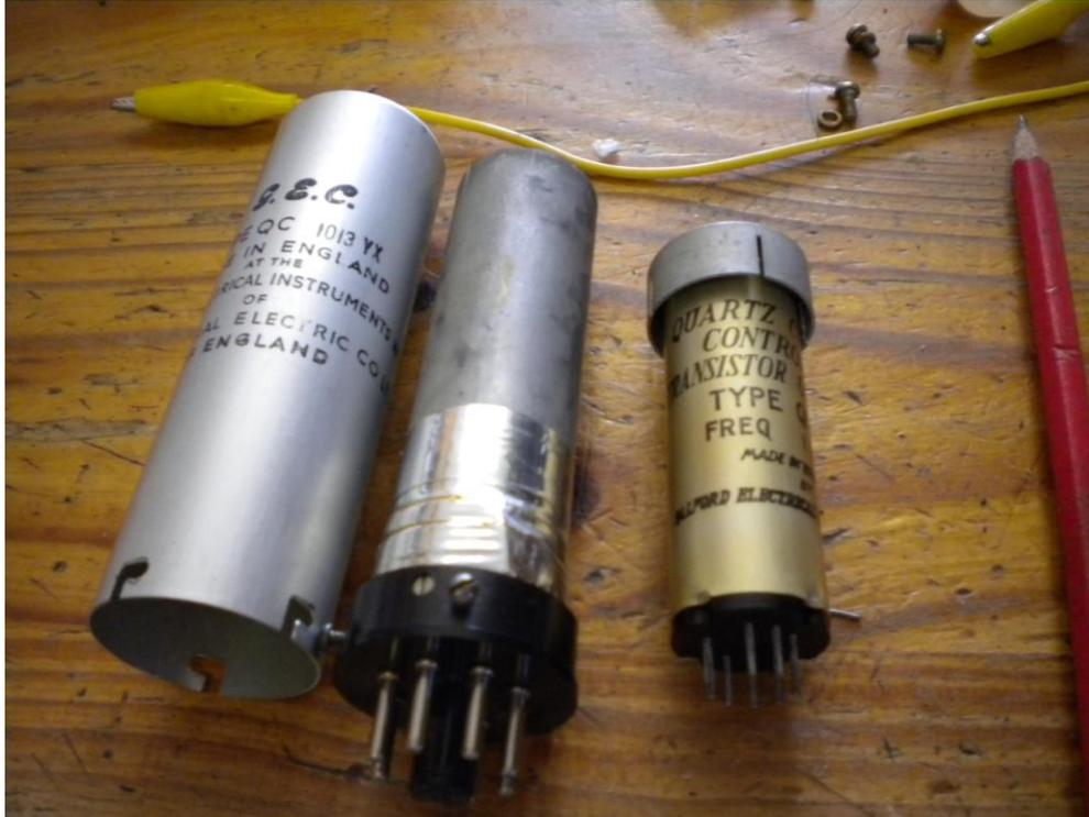
Now in my case the pins to the 9 pin B9A socket were badly oxidised so hopefully a good clean will get it working but NO it didn't . So investigation further dedeed. With a small screwdriver ease up the 4 crimps about the base of the inner can.
