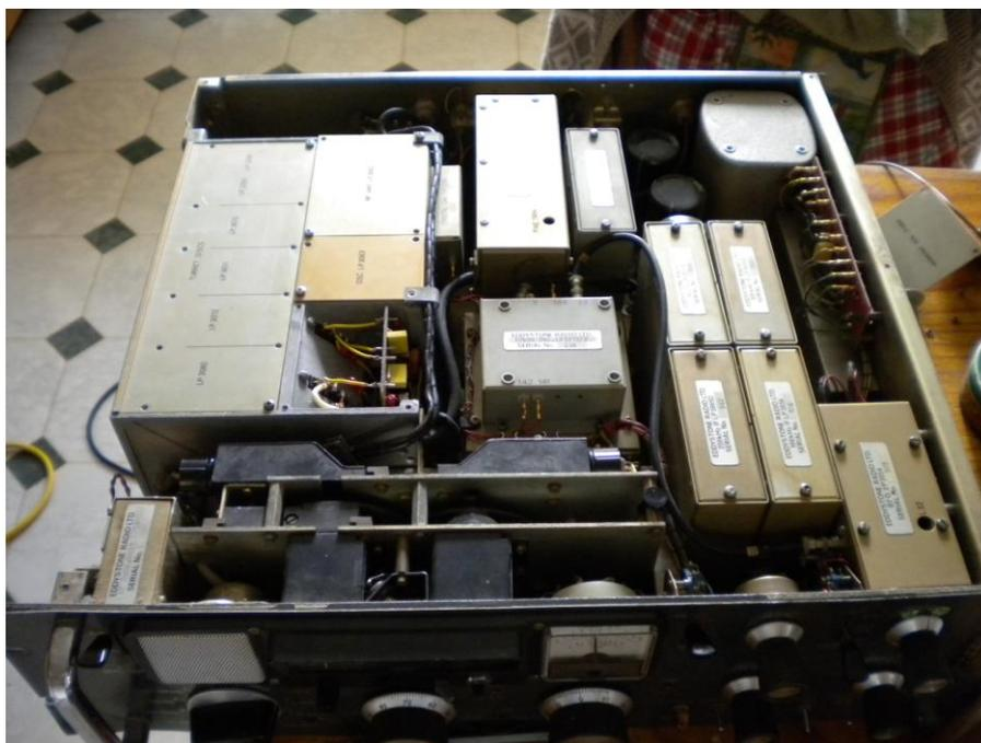
This receiver was obtained from a clear out at a local radio club as being totally not working at all. Subsequent examination and basic repairs got the basic set working but not the Stabilised loop system used on ranges 1-4 ie 1.6 Mhz to 30 Mhz.
