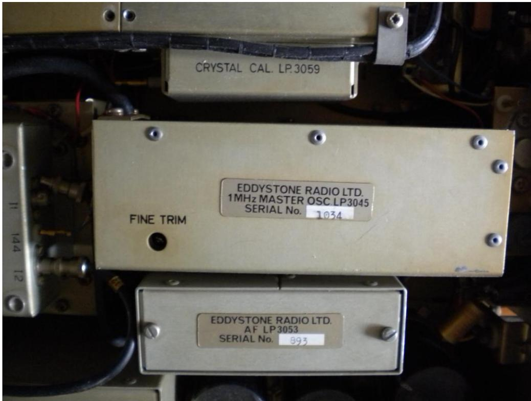
Now the master Osc unit looks formidable however after examining the manual there are only four voltage connection and two RF outputs.
