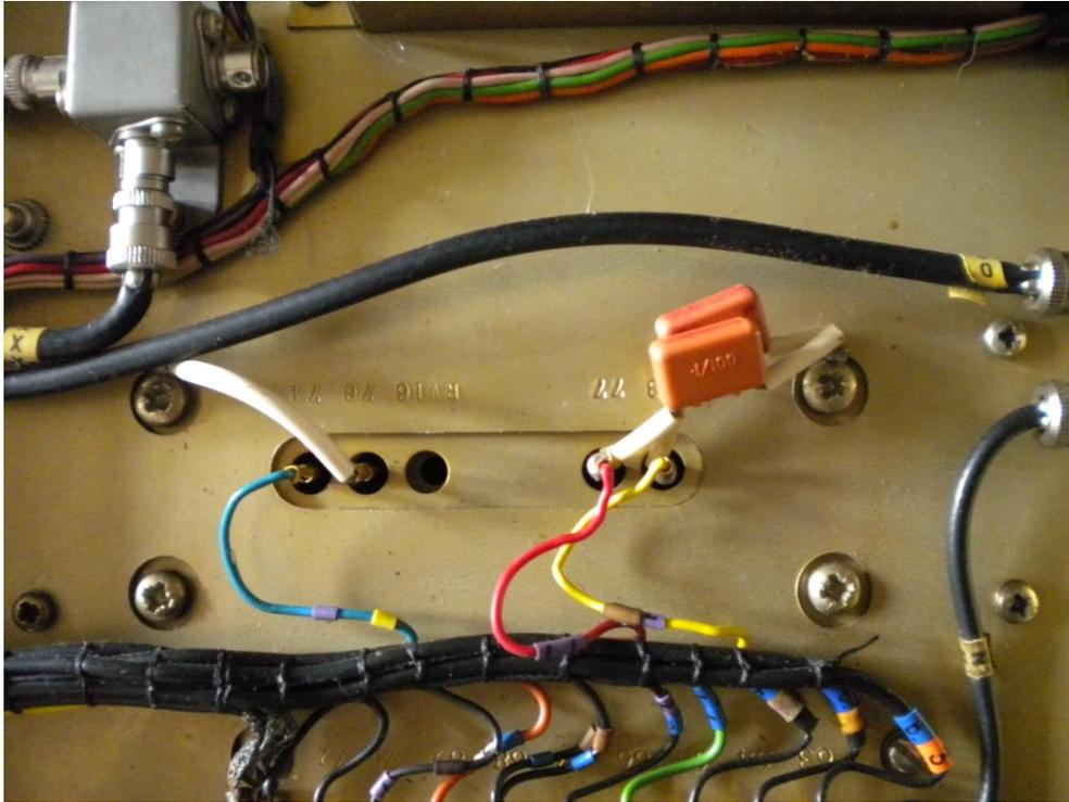
Therefore there was no alternative but to extract the module for further examination. Reading the manual the voltage connections were unplugged from the base of the unit. Coax plug "I" was unplugged and coax G was further unsoldered from within the RF box. The 4 x 6 Ba screw holding it in place was unscrewed and the module came out no problem.
