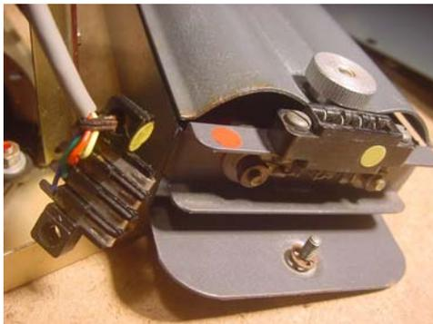
battery holder, or else another connector type would need to be fitted. This did not appeal to me much - then I thought 'why not build the supply inside the battery holder, thus preserving the original appearance of the set and without dismantling the holder?' I set about doing this with the intent of making the supply such that no modifications were needed to the battery holder or set whatsoever... interested? – then read on.
