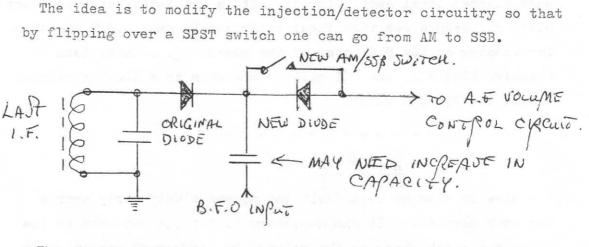
The above circuit is not original and was originally seen as a mod for a 'surplus model' receiver, non-Eddystone of course.
